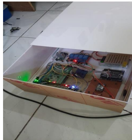
Fig. 6. Smart bird cage implementation design
